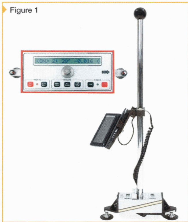
Figure 1 Apparatuses for measuring joint stability. These devices test the differential deflection of adjacent slab panels.
